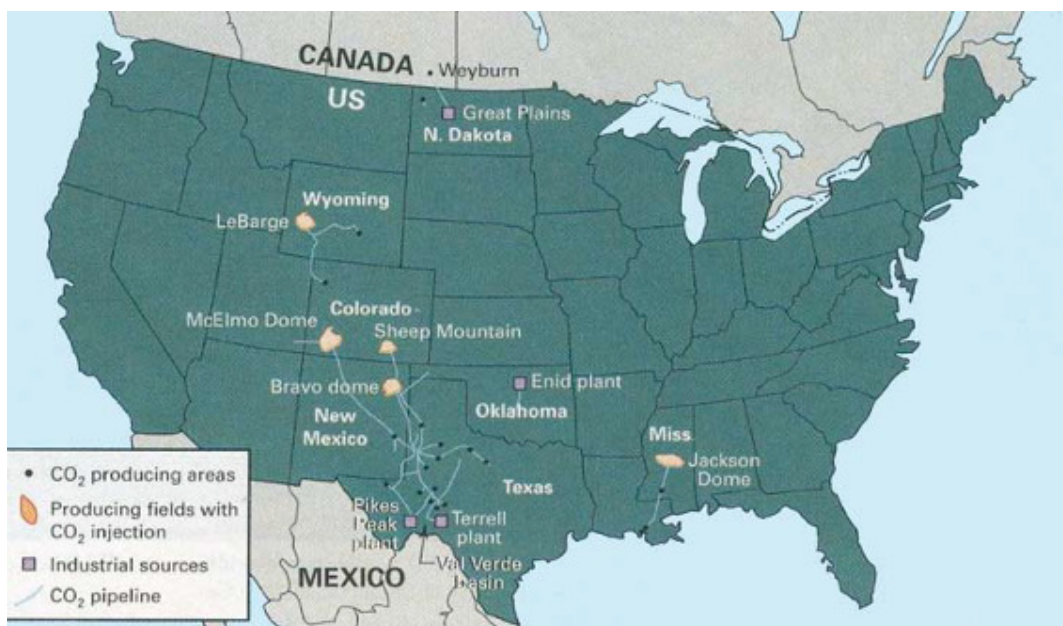
Figure 5.1 CO 2 pipelines in North America. (Courtesy of Oil and Gas Journal)..
